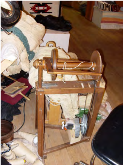
Assorted equipment (including Lisa's "real" walking loom and her "for fun" 4-shaft workshop loom) has crept into nooks and crannies in the gallery. This bulky head spinner is powered by a sewing machine motor.
