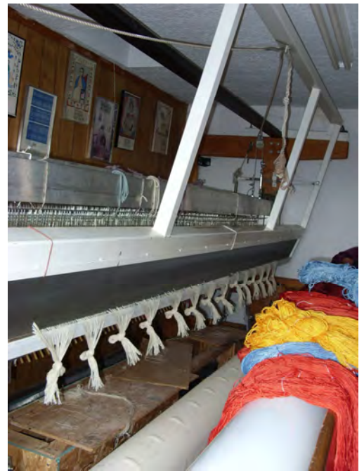
Irvin's really big loom. Lisa thinks it's a 12-foot weaving with. Sheds are changed with a modified electric garage door opener.
