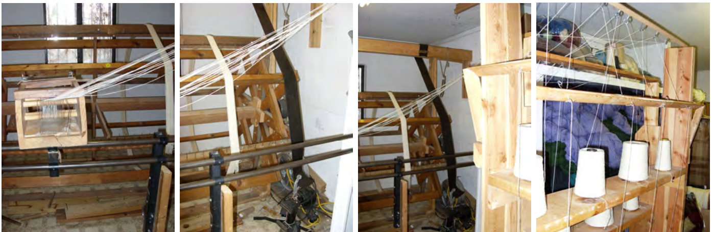
Warps are wound sectionally from a creel over a ceiling hook, through a tension box, and onto an industry-style warping wheel. The warp is then wound from the wheel onto a warp beam, which is held on brackets in front of the wheel. The warp for multiple tapestries is put on the beam at the same time. In the photos, the creel is rotated 90 degrees to allow access to the room; when in use, it would be parallel to the wheel. The warping wheel is HUGE!
