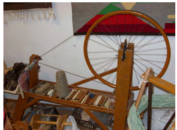
Hand-cranked bicycle-wheel bobbin winder
